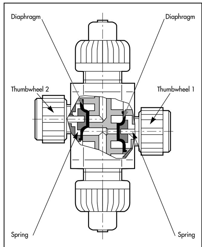
**Note :** This valve is calibrated in the plant in compliance with the service conditions communicated by the customer at the time of order. By default, calibration is 2 bar for the loading valve function.
